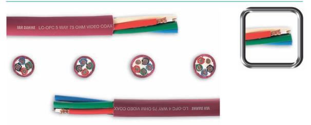
Van Damme Red Series Video multicores are 4 and 5 way versions of the Van Damme standard 75 Ohm coaxes. Designed for use in the Presentation and Broadcast industries, they are commonly used for the transmission of video signals such as RGBHV and RGB Sync over longer distances - up to 100 metres for analogue video signals. They are flexible but also very robust and are ideal for multiple rig and de-rig situations due to the attention paid to their construction, overall diameter and weight.
