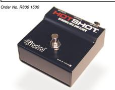
The Radial Hot Shot DM-1 is a combination microphone signal splitter and mute switch that allows the vocalist to depress a footswitch to mute his mic and redirect the signal to the monitoring system and/or intercom. This 100% passive floor-box is equipped with XLR mic input, momentary footswitch, direct and switched XLR outputs.
