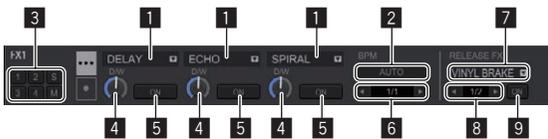
Single mode: One beat FX and one release FX can be selected per effect unit, and beat FX has multiple adjustable parameters.
